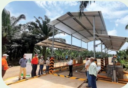
Foot bath and tire bath for Fusarium TR4 prevention through the disinfection of vehicles and hygiene at the entrance of people
